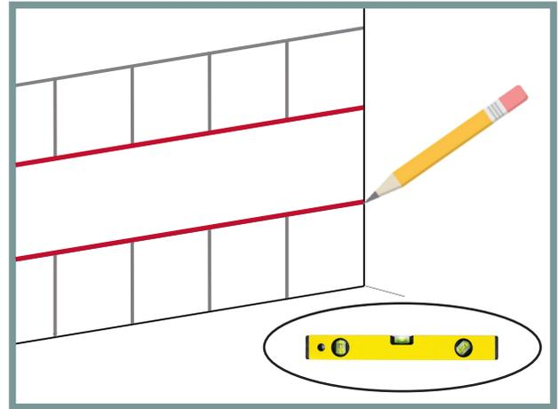
4. Draw a level line at 34 1/2" from the highest point of your floor and another level line at 54 1/2" from the same point. Install the top of the base cabinets level with the 34 1/2" line by using the adjustable legs to level the cabinets. Install the bottom of the wall cabinets level with the 54 1/2" inch line.
