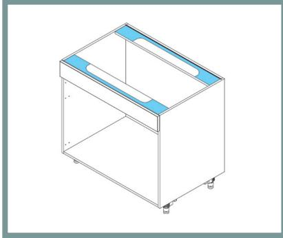
When installing a sink or cooktop, trimming the top support rails may be necessary. Using the template supplied by the sink or cooktop manufacturer, cut the top rails as required using a jigsaw.
