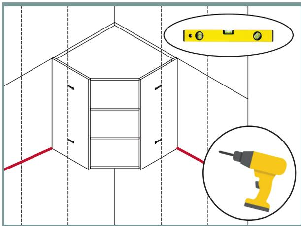
5. Starting with the corner wall cabinet, install (x4) 2 1/2" cabinet screws through the fastening strips on the cabinet into the wall studs. Be sure to check for level before fastening the cabinet into place.
