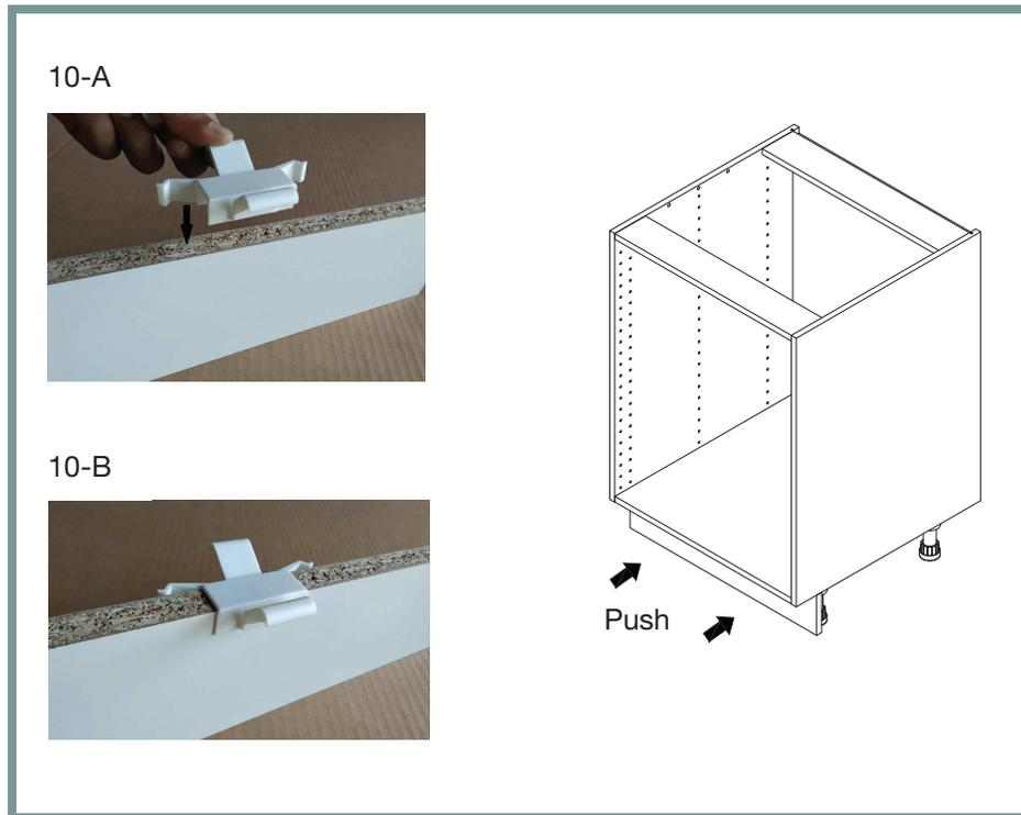
10. To install the toe-kick clips, push the clip onto the top of the toe-kick as shown in step 10-A and step 10-B. To install the toe-kick, insert the top first and then push at the bottom to make a tight fit.
