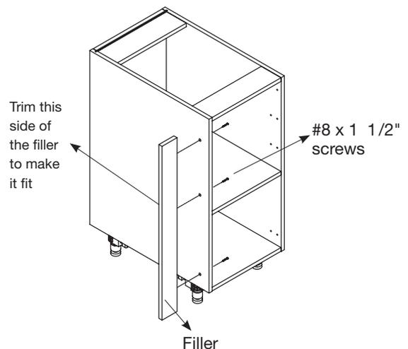
Install the remaining base cabinets by aligning the front of the cabinet edges. Clamp the cabinets together and attach using the 1 1/8" screws. Level the cabinet, adjust as required, and attach to the wall studs using 2 1/2" screws through the hanging rail located at the top of the base cabinet. After inserting the screws remove the clamps.
