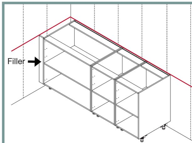
11. For designs without a corner cabinet, start with the first cabinet leaving space for a filler, as per your plan.
