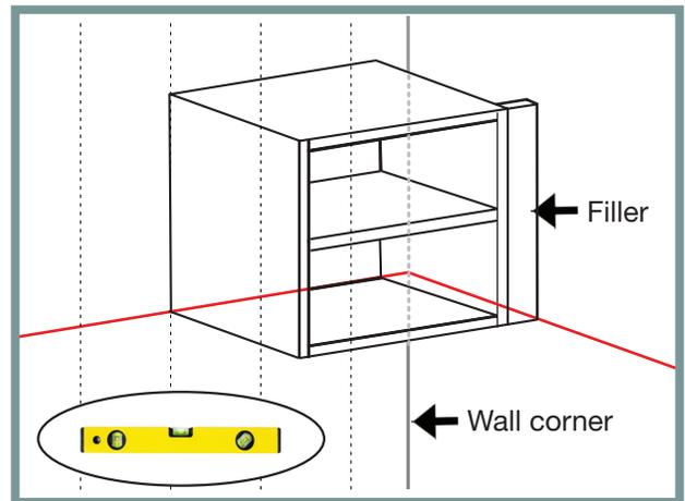
6. If you do not have a corner, start with the end closest to a wall, making sure to leave room for the required filler, as per your plan.
